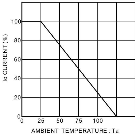
Fig. 4 Derating curve
