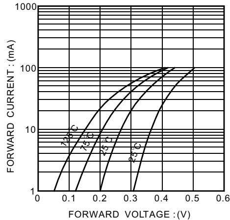
Fig. 1 Forward characteristics
