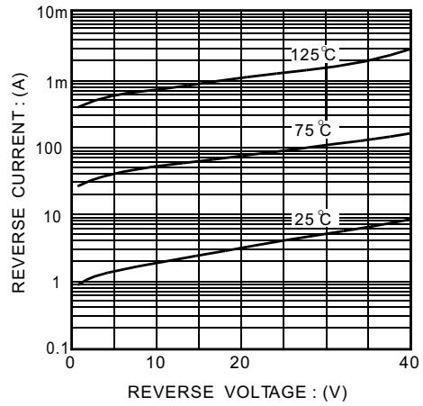
Fig. 2 Reverse characteristics
